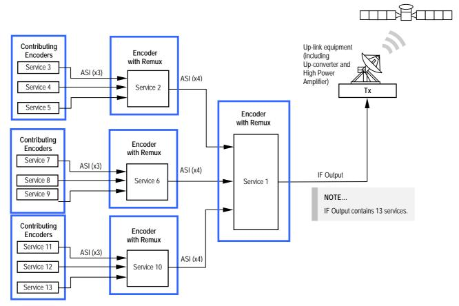
Figure 3.5: Block Diagram – Two Stages of Remultiplexing
